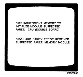
Figure 8-28.—Examples of test results from an external
